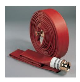
Features specially formulated high grade synthetic rubber extruded through an all polyamide woven jacket to give a non-kinking construction and the best rubber-to-textile adhesion that modern technology can achieve.
